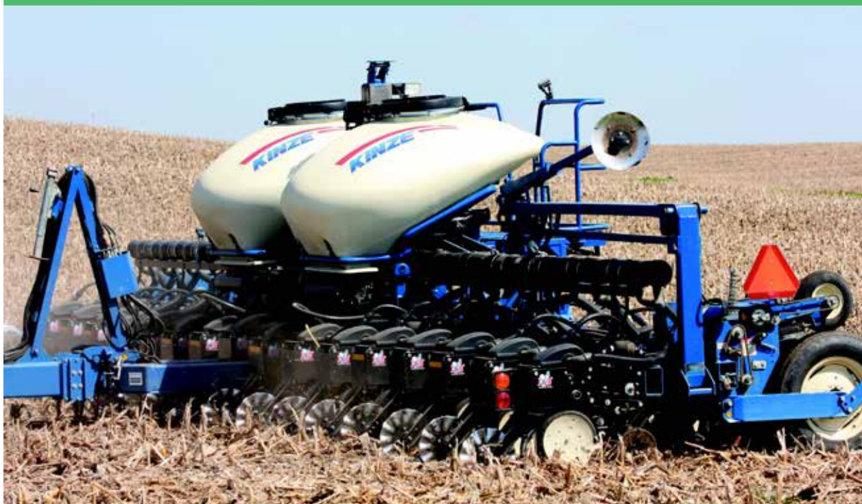
Granular fertilizer or herbicide attachment planter
