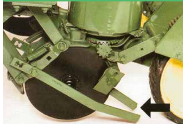
Knife coverer = knife covering attachment پوشاننده کاردی
