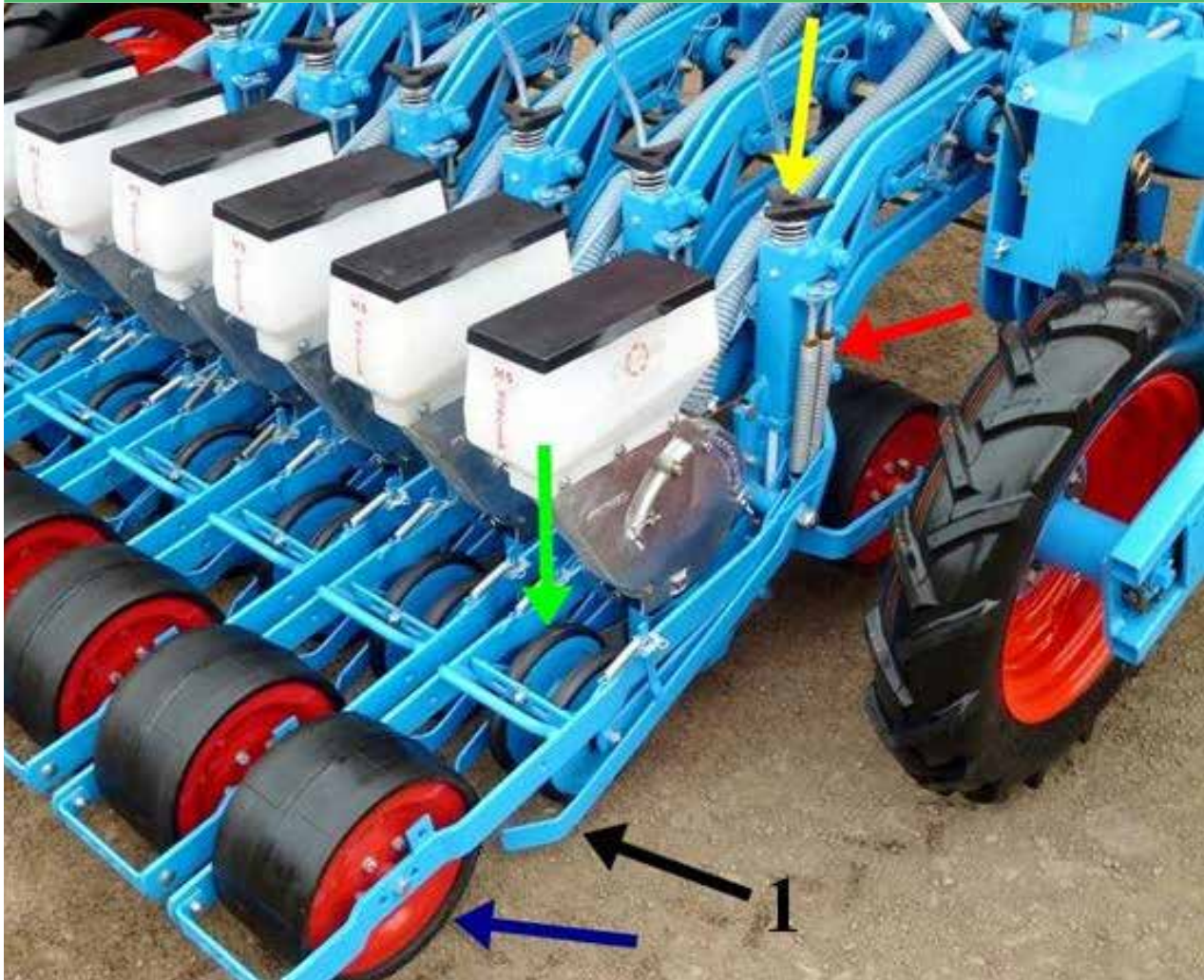
Knife coverer = knife covering attachment پوشاننده کاردی
