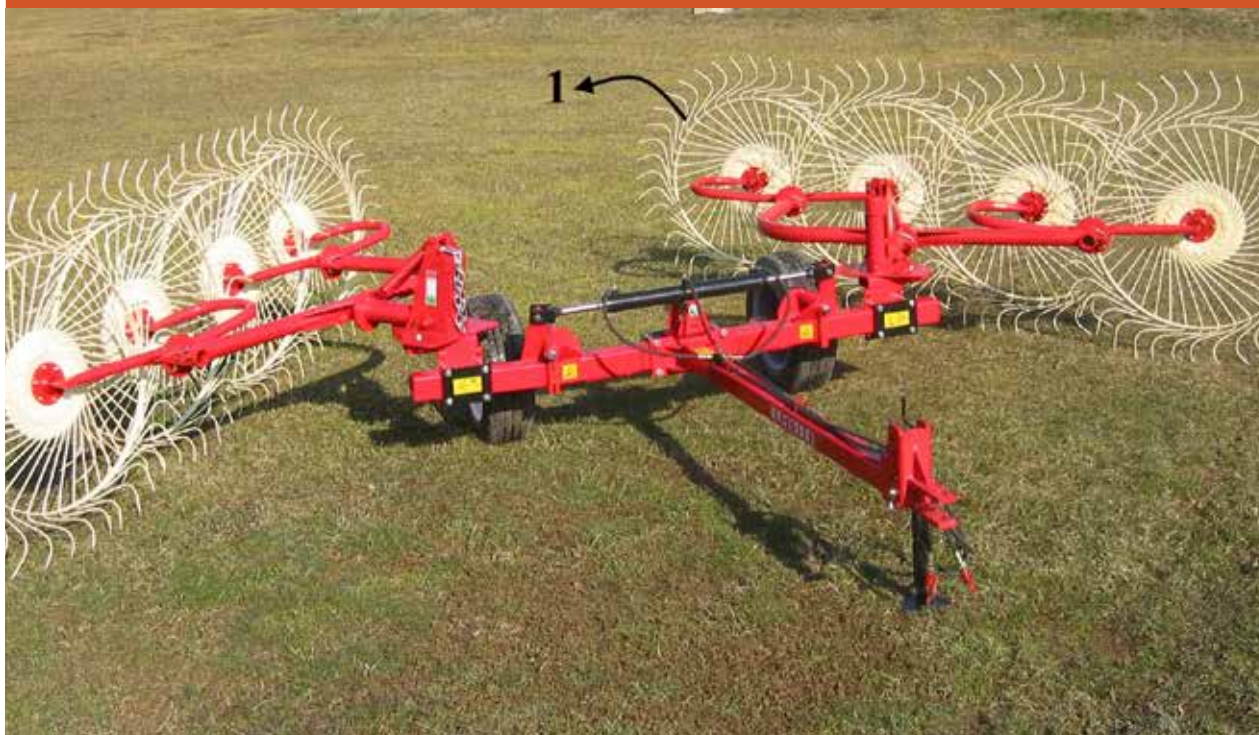
Wheel rake (1-Finger wheel)
