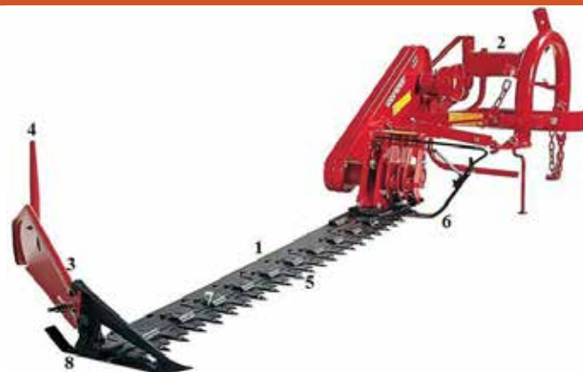
Cutter bar mower (1- Cutter bar 2- Frame 3- Grass board = swath board 4- Grass stick 5- Guard = finger 6-Inner Shoe 7- Knife clip = Knife keep 8- Outer shoe)
