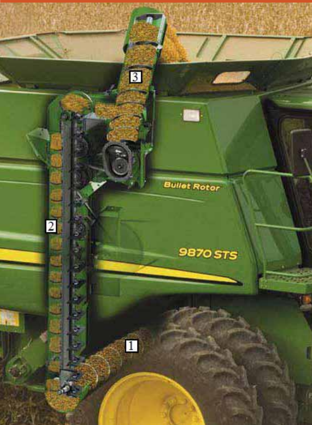
Handling unit (1- Grain auger 2- Grain elevator 3- Upper grain auger)
